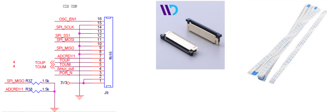
Figure 3 16-pin, 0.5mm pitch FFC connector for ULS24 Module
