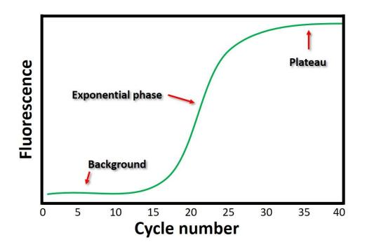
Figure 1 qPCR fluorescence curve. The fluorescence emission level from the sample is at some baseline level prior to amplification. It will then monotonically rise and saturate at some higher level.
