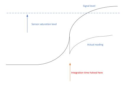
Figure 2 Dynamically adjust integration time to avoid signal saturation.
